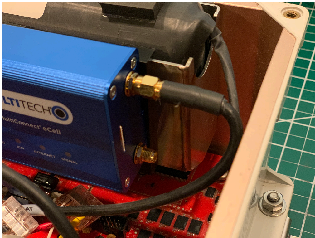
SMA connector from PCB - connects to CELL
