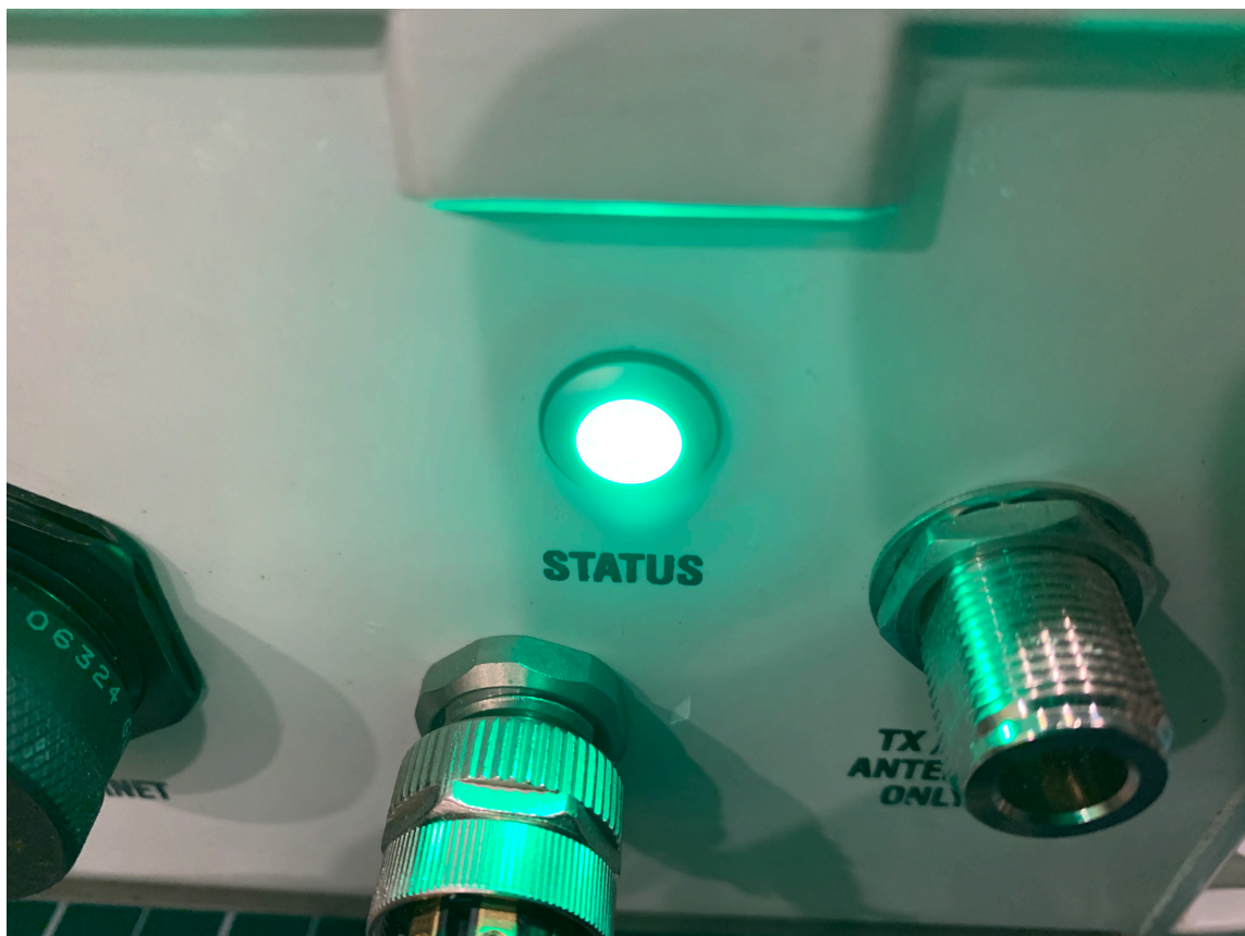
Status light, external power: steady on battery: flashing
