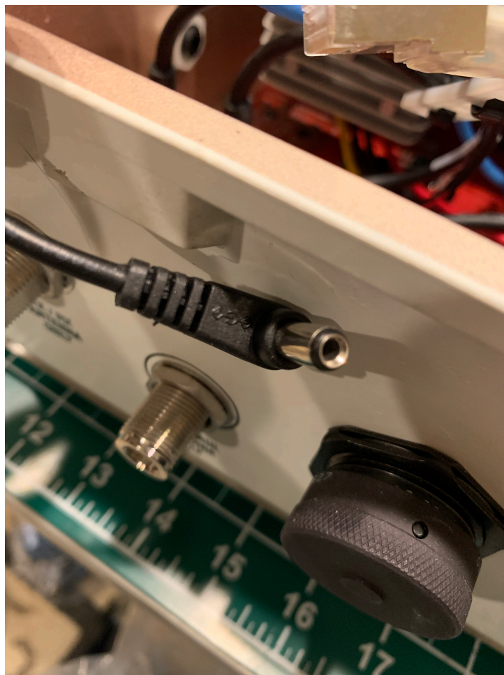
e-cell power plug - positive center - 12 volts
